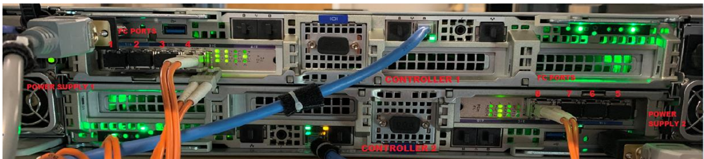
Rear view of V1000 XE or 4 port V1000 SE. V1000 SE has option of 2 ports
