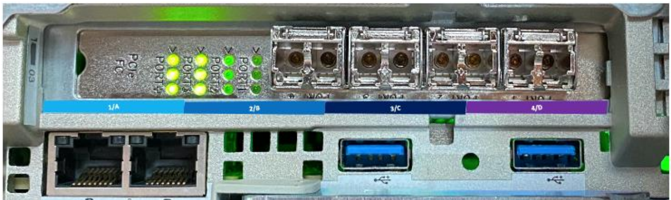
Fibre Channel Interconnect (Controller). The QV1020 has option of 2 ports
