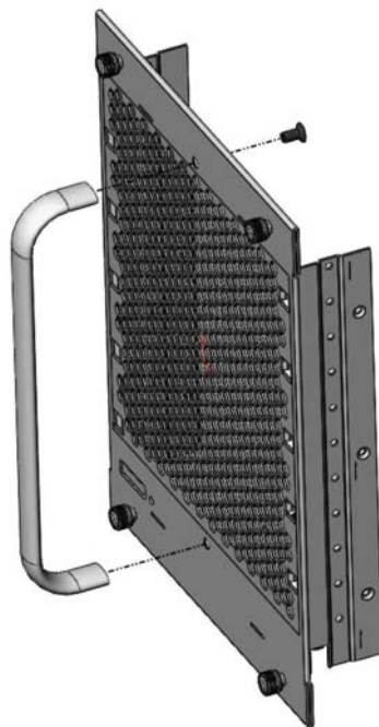
FIGURE 170 Handle removal
