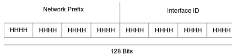
FIGURE 34 IPv6 address format
